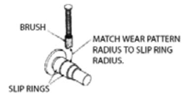
If the original brushes are being used, then the wear pattern of the brush must be matched with the radius of the slip ring (Fig. 5).
