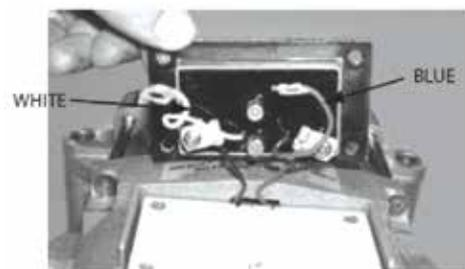
**CAUTION:** All screws that may fall into the regulator holder must be removed at this time to prevent them from falling into the slip ring cavity through the brush openings.
