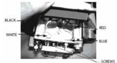
3) Install the BLUE and WHITE regulator leads with the #10 square head screws and #10-32 self-locking nut to the inside of the regulator holder (Fig. 6).
